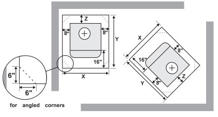
NOTE: In Canada, floor protection must extend 18" (450mm) to the front and 8" (203mm) to each side and back of the stove.
